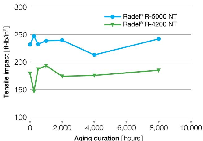
**Figure 10:** Dynatup instrumented impact after aging in 90 °C water
