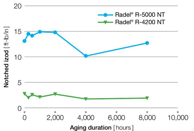
**Figure 9:** Tensile impact after aging in 90 °C water
